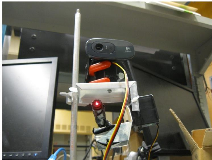
Figure : Completed Laser Turret
