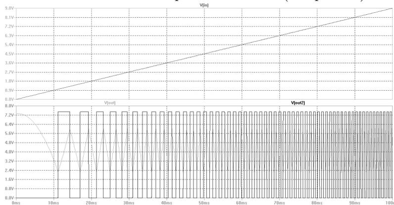
FIGURE 6. VCO Graph of Control Voltage vs Frequency.
