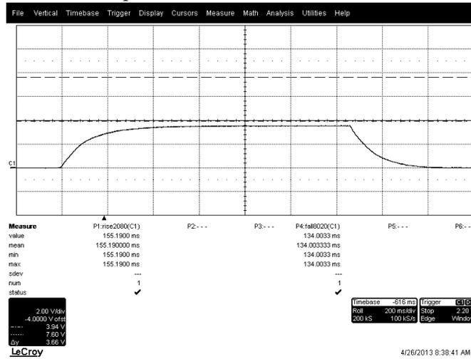
FIGURE 11. Measured Outputs from AR Envelope Generator to On-Off Gate ( $V_{on} = 4.5V$ ), RV3 and RV4 set to minimum position.
