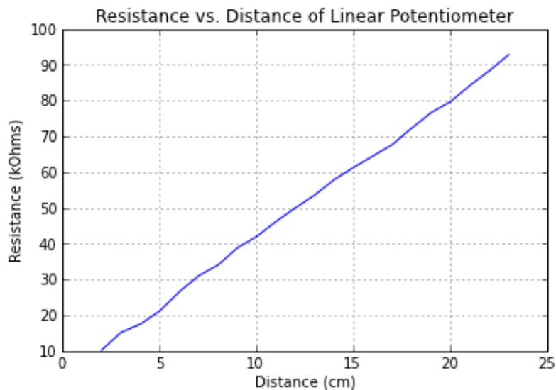
**2.1. Input Stage.** The input stage of our synthesizer is a ribbon controller. This type of controller is essentially a linearly actuated potentiometer. We used a strip of conductive plastic, often found protecting electronics from ESD during shipping, mounted to a piece of wood and a wiper suspended above it to
