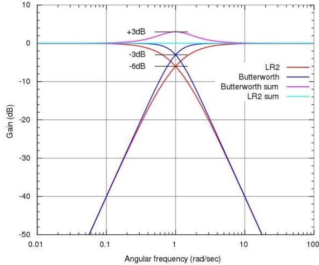
$$(13) \quad \left| \frac{V_{out}}{V_{in}} \right|_{\omega=\omega_0} = \sqrt{\frac{R_2 * C_2}{R_1 * C_1}} * Q = \sqrt{\frac{RC}{RC}} * Q = Q = .5$$
