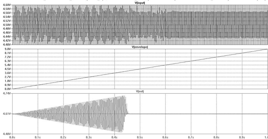
FIGURE 8. VCA Output w/ Sine Input (200mV peak to peak). Envelope provided by AR Envelope Generator. Over Whole Envelope
